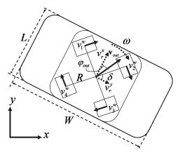
Fig. 10. An omni-directional platform with wide body
