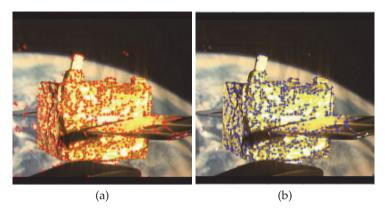
Fig. 11. Feature points extracted by the Harris corner detector without (a) and with employing color information (b).
