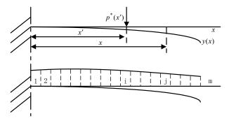
Fig. 2. Deformation of the roll from an arbitrary load distribution
