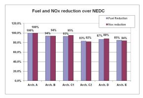
Fig. 17. Fuel consumption and NOx emissions reduction over NEDC for different diesel hybrid architectures with a "NOx cut" strategy.
