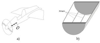
Fig. 1. (a) an example of extensive cutout in the airframe structure; (b) isolated, critical fragment of the structure
