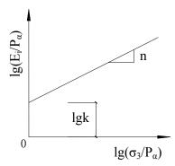
Fig. 3. The relation between  $\lg(E_i/P_a)$  and  $\lg(\sigma_3/P_a)$
