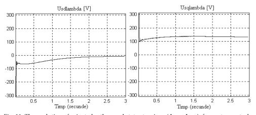
Fig. 11. The evolution of oriented orthogonal stator tensions (**d.c. values**), for vector control with robust-adaptive rotor flux estimator ( $\omega_m^* = 157 \text{ rad/s}$ ).
