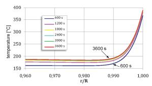
Fig. 12. Radial temperature at different time instants for plane FE model.
