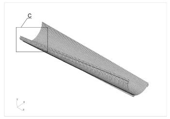
Fig. 12. Reinforced structure - version 2 - continuous connection of surface and stringers. Local post-buckling deformation.
