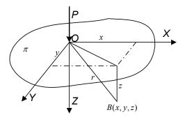
Fig. 3. Semi-infinite body model
