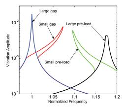
Fig. 8. Effect of N<sub>0</sub> on the dynamics of the system with variable normal contact load.
