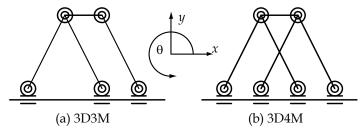
Fig. 2. 3-DOF planar parallel mechanisms
