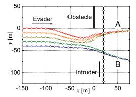
Fig. 15. Trajectory of evader with IAFB starting from different initial positions.
