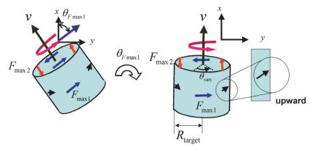
Fig. 7. Schematic diagrams for the estimation of the rotational axis.
