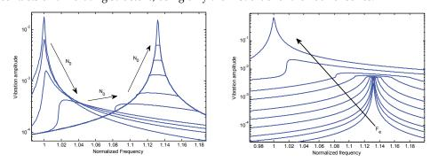
Fig. 5. Effect of  $N_0$  (left) and of  $F_E$  (right) on the dynamics of the system
