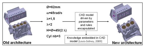
Fig. 2. Parametric design method on an automotive Power Unit
