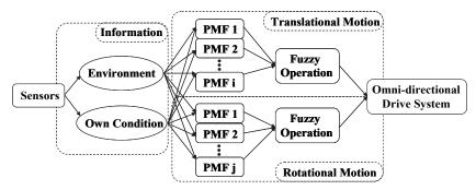
Fig. 4. A concept of fuzzy potential method considering translational and rotational motion with an omni-directional platform
