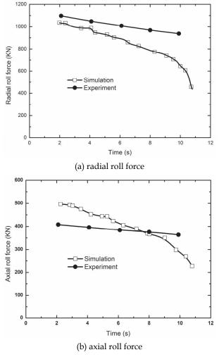
Fig. 6. Measured and predicted variations of the roll forces at the stable rolling stage
