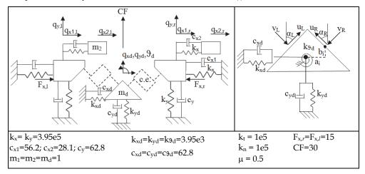
Fig. 12. Multiple dof description, blade-to-blade friction damper application
