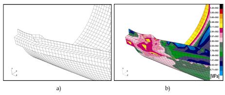
Fig. 11. Form of post-buckling deformation; a) area of C detail in actual scale; b) effective stress distribution on external surface according to von Mises' criterion.
