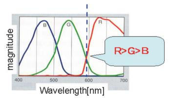
Fig. 6. Schematic representation of spectral response curve of the panel.
