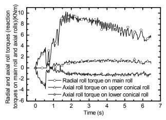
Fig. 15. Variation curves of the radial and axial roll forces during the radial-axial ring rolling process
