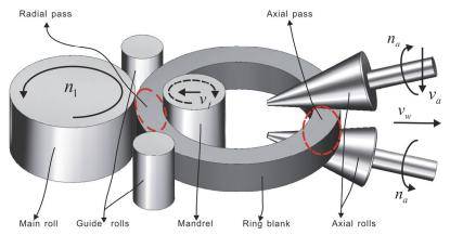
Fig. 1. Forming principle of radial-axial ring rolling
