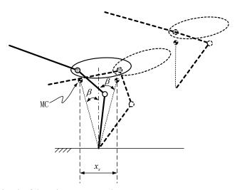
Fig. 2. Motion sketch of the robot in stance phase
