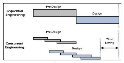
Fig. 1. Concurrent engineering approach for time saving in the design process
