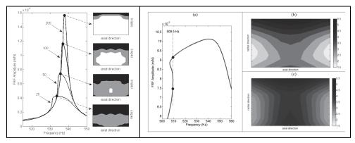
Fig. 23. Effect of the damper mass on the contact status (left). Different distributions of static normal load in case of coupled static/dynamic calculation (right).
