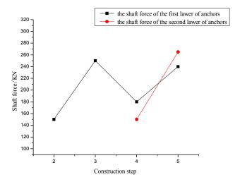
Fig. 18. Axial force of soil anchor curve
