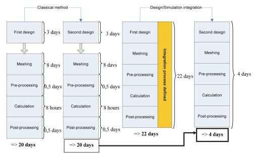
Fig. 6. Classical method vs design/simulation method
