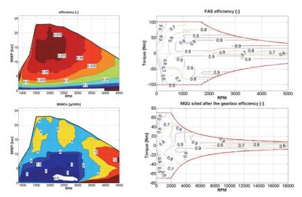
Fig. 15. Performance Maps – Left: Engine Efficiency and BSNOx maps. Right: MGUs efficiency maps.
