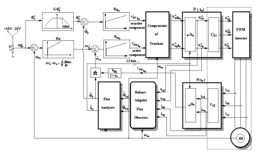
Fig. 8. Modelling of the closed-loop vector control system
