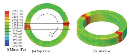
Fig. 10. Stress distribution contour of the rolled ring
