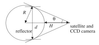
Fig. 3. Geometric relationships between the satellite and the size of the reflector.
