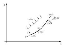
Fig. 5.4 The forces acting on a short segment of SCR
