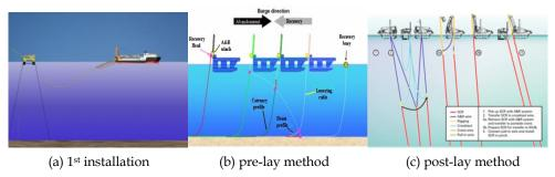
Fig. 5.3 SCR installation methods
