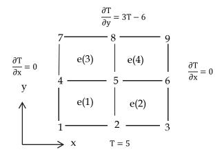
Fig. 7. Two-dimensional region divided into four square elements with boundary conditions When combines and applied the specified boundary condition, the final system equation becomes 6 by 6 matrix as
