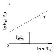
Fig. 9.  $\lg(E_{ur}/P_a) \sim \lg(\sigma_3/P_a)$  relation curve
