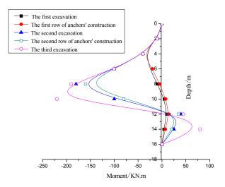
Fig. 17. Moment of steel sheet pile curve graph
