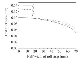
Fig. 16. Effect of transverse friction on strip shape
