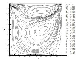
Fig. 11. Horizontal velocity contours for driven cavity problem for Reynolds 100
