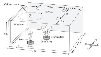
Fig. 5. Room model considered in our numerical analysis. Ambient light includes sunlight (through the window) and four incandescent lamps.
