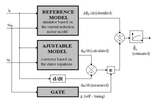
Fig. 4. The structure of the adaptive flux observer
