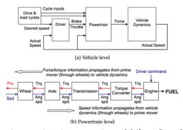
Fig. 3. Information flow in a quasi-static powertrain model (from Guzzella & Sciarretta, 2007).
