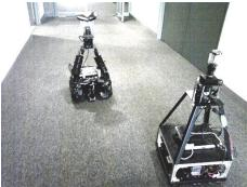
Fig. 1. An omni-directional platform of a prototype robot (left), a situation that the robot needs to avoid the other robot (right)
