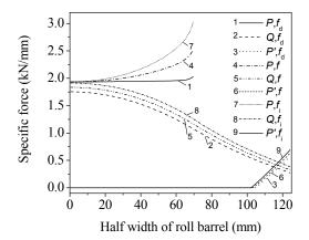
Fig. 17. Effect of transverse friction on specific forces
