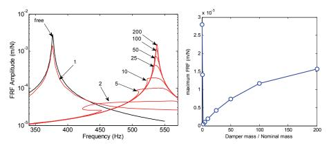
Fig. 22. Effect of the damper mass ( $m_d = n \times m_{nom}$  with n = [1:200].): FRF curves (left) and optimization plot (right).
