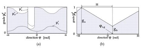
Fig. 8. PMFs for rotational motions:  $\mu_o^r$  is a PMF for an obstacle (a),  $\mu_g^r$  is a PMF for a goal (b)
