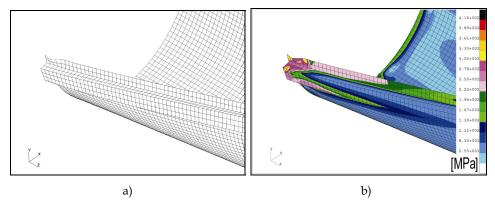
Fig. 13. Form of post-buckling deformation; a) area of B detail in actual scale; b) effective stress distribution on the external surface according to von Mises' criterion.
