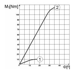
Fig. 4. Representative equilibrium path: torsion angle versus torque moment: 1 - shell without reinforcement, 2 - structure with stiffeners
