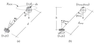
Fig. 4. (a) Link geometry used to compute the sunlight power received by a conventional single-channel receiver. (b) Link geometry employed to compute the artificial light power received by single-channel imaging receiver.
