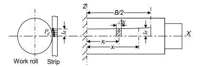
Fig. 4. Flattening between the work roll and strip
