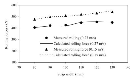
Fig. 19. Effects of the rolling speeds and strip widths on rolling forces
