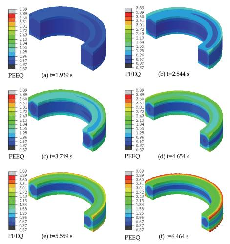
Fig. 11. Equivalent plastic strain (PEEQ) distribution contour under different time during the radial-axial ring rolling process
