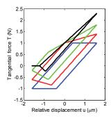
Fig. 7. 1D relative displacements and variable normal load: contact model (left) and typical hysteresis cycles (right)
