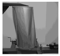
Fig. 19. Advanced post-buckling deformation,  $M_t = 60 \text{ Nm}$ .  $M_t = 60 \text{ Nm}$ . (structure with three stringers)
