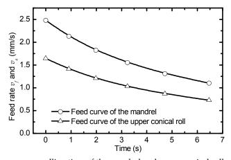
Fig. 8. Feed curves versus rolling time of the mandrel and upper conical roll
