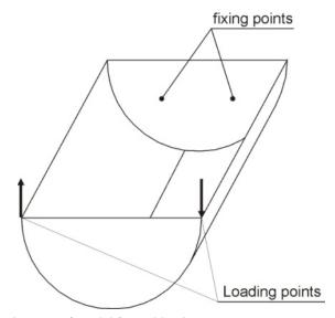
Fig. 25. Schematic diagram of model fix and load
