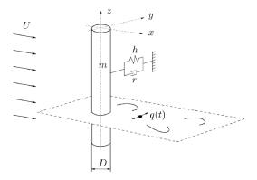
Fig. 4.3 Wake oscillator model
