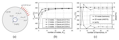
Fig. 4. (a) Thermal layout used in comparative test (material thermal conductivity is  $\lambda$ =50 W/mK); (b) converge rate: trend of calculated maximum temperature vs. number of nodes in the mesh, for different element types; (c) results accuracy vs. number of harmonics H.
