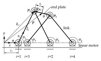
Fig. 5. Kinematic model of the 3-DOF PLM
