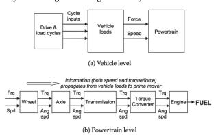
Fig. 1. Information flow in a kinematic or backward simulator (from Guzzella & Sciarretta, 2007).
