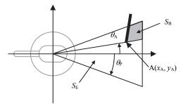
Fig. 13. Vehicle in body fixed coordinate system.
