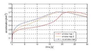
Fig. 13. (Effect of different smoke maps) Acceleration vs. time. Manoeuvre: tip-in from 60 km/h, VI gear.
