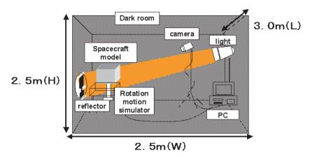
Fig. 1. Schematic representation of the in-space lighting simulator.
