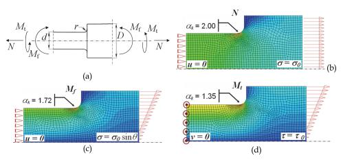
Fig. 6. (a) Analysed geometry with different applied loads (N axial,  $M_f$  bending,  $M_t$  torsion); (b), (c), (d) plane FE models used in semi-analytical approach, with loads and constraints (values of  $\alpha_k$  indicate the numerically calculated stress concentration factors)
