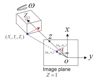
Fig. 8. Relationships between the rotational motion of the target and optical flow.
