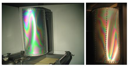
Fig. 23. Optical effect distributions: a model with 3 stringers (left), a model with 5 stringers (right)
