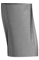
Fig. 33. Structure reinforced by 7 stringers – comparison of deformation forms obtained as the result of experiment (left) and nonlinear numerical analysis (right) – stringers reproduced with brick elements
