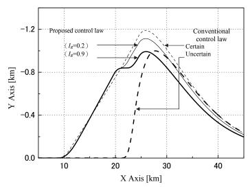
Fig. 10. Avoidance trajectory of the cases with/without proposed control law using uncertain parameters ( $I_P = 0.25$ ).
