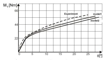
Fig. 28. Comparison of representative equilibrium paths: model1 — stringers of 3D elements; model2 — stringers of beam elements
