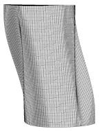
Fig. 32. Structure reinforced by 5 stringers – comparison of deformation forms obtained as the result of experiment (left) and nonlinear numerical analysis (right) – stringers reproduced with beam elements
