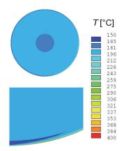
Fig. 10. Temperature distribution in work roll after 1800 s given by plane FE model.
