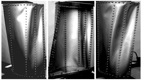
Fig. 21. Advanced post-buckling deformation pattern (structure with 7 stringers), Mt=110 Nm
