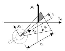
Fig. 12. Vehicle in ground fixed coordinate system.
