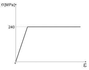
Fig. 7. Stress-strain relation of idealised material.
