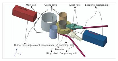
Fig. 4. The coupled thermo-mechanical 3D-FE model for the entire radial-axial ring rolling process
