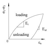
Fig. 8. Loading and unloading relation curve
