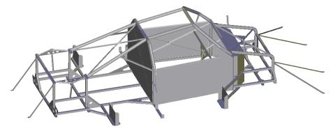
Fig. 13. CAD model of the E-Sphyra's frame
