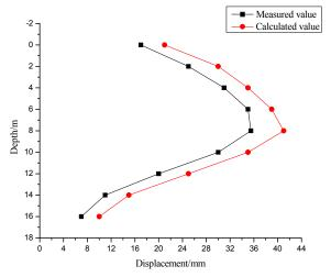
Fig. 15. Final calculated and measured values of horizontal displacement curve graph
