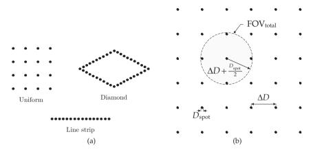
Fig. 2. (a) Transmitter pattern geometries proposed in the literature. (b) Transmitter pattern used in our analysis.
