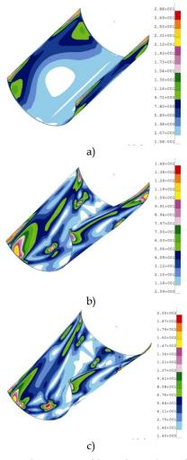
Fig. 29. Stress distributions according to Mises' hypothesis: (a model with stringers represented by beam elements) a) 25% load — middle layer; b) 70% load — middle layer; c) 100% load — middle layer
