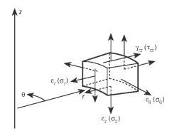
Fig. 2. Strains and stresses involved in an axisymmetric analysis
