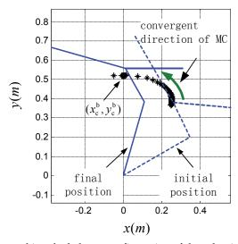
Fig. 3. Simulation for searching the balance configuration of the robot in stance phase
