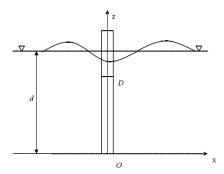
Fig. 4.1 Small scale straight cylinder coordinate system
