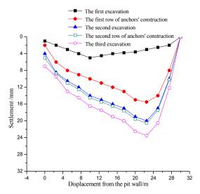
Fig. 16. Ground settlement behind pile curve graph
