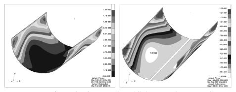
Fig. 26. Comparison of stress distributions in the middle layer according to Mises' hypothesis obtained for the discrete joints model (left) and the continuous joints model (right)
