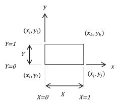
Fig. 3. Two-dimensional linear rectangular element.
