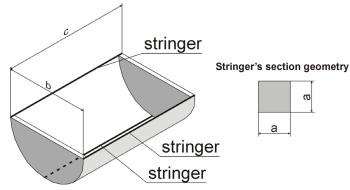
Fig. 15. Schematic geometry of the structure (a=10mm)
