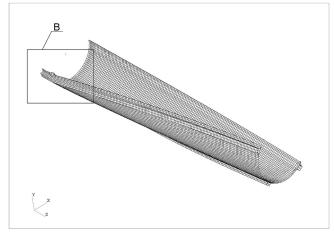
Fig. 10. Reinforced structure -version 1- riveted joint of the surface with the stringer. Local post-buckling deformation.
