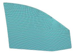
Fig. 11. Mesh of a window for FE simulation
