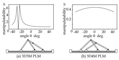
Fig. 6. Singularity analysis of the parallel link mechanisms
