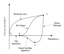
Fig. 2.1 Typical P-y curve
