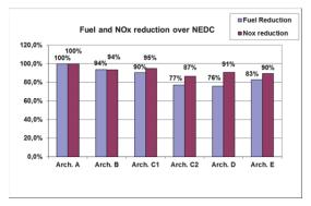
Fig. 16. Fuel consumption and NOx emissions reduction over NEDC for different diesel hybrid architectures with a "conventional" energy management strategy.
