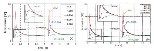
Fig. 13. Temperature time history for points at different radial depths, along the same angular position. (a) plane and (b) harmonic FE model.
