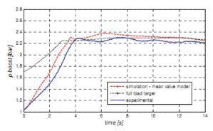
Fig. 12. Boost pressure vs. time. Manoeuvre: tip-in from 40 km/h, IV gear.
