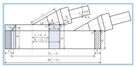
Fig. 7. Position variation of the upper conical roll before and after rolling
