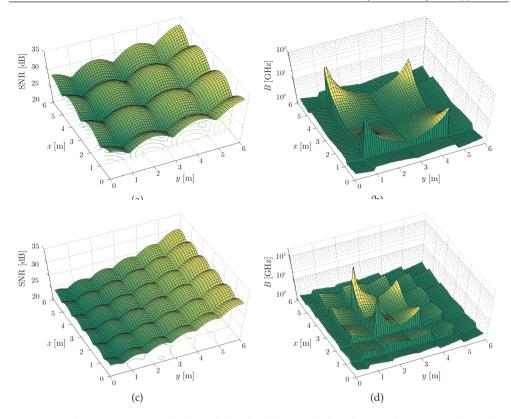
Fig. 6. Signal-to-noise ratio and channel bandwidth spatial distributions for CSCR links and SCIR links. (a) SNR for CSCR links. (b) Channel BW for CSCR links. (c) SNR for SCIR links. (b) Channel BW for SCIR links. CSCR links employ a MBT with 16 beams and a receiver with a FOV $_{\rm total}=45^{\circ}$ . SCIR links uses a MBT with 36 beams and a receiver with a FOV $_{\rm total}=30^{\circ}$ . A transmitter power  $P_{tx}=200$  mW is assumed in all cases.
