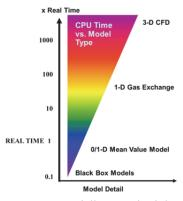
Fig. 5. Flowchart of the main engine modelling methodologies, showing model detail vs. computational time.
