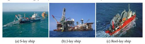
Fig. 5.1 Three pipelay ships
