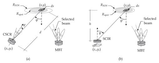
Fig. 3. (a) Link geometry used to compute the received power signal in a conventional single-channel receiver. (b) Link geometry used to compute the received power signal in a single-channel imaging receiver.
