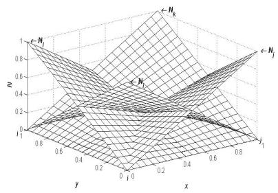
Fig. 4. Two-dimensional rectangular linear element shape functions distribution.
