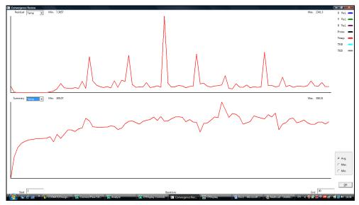
Fig. 6. Convergence of the nodal temperature after 90 iterations
