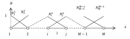
Fig. 5. System of elements shape function and nodes
