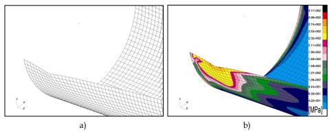
Fig. 9. Form of post buckling deformation; a) area of A detail in actual scale; b) effective stress distribution on external surface according to von Mises' criterion.
