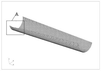
Fig. 8. Post buckling deformation. Structure without stringers
