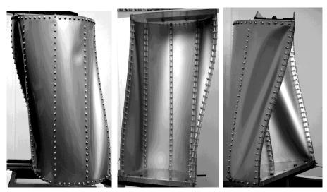
Fig. 20. Advanced post-buckling deformation phase (structure with 5 stringers),  $M_t = 75$  Nm.
