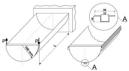
Fig. 2. Installation, loading device, and dimensions of the cross section.
