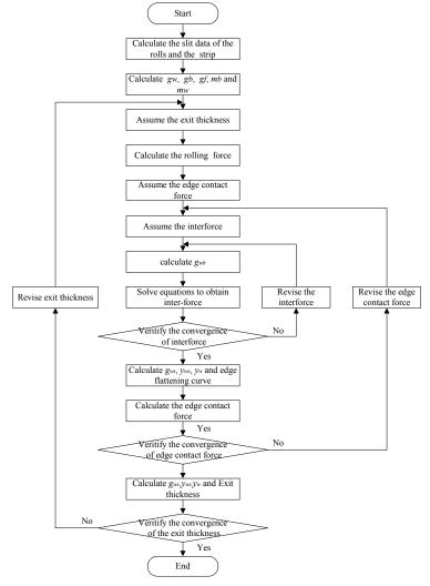
Fig. 9. Flow chart of the roll and strip deformation and strip shape calculation
