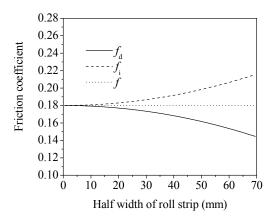
Fig. 15. Distribution of friction coefficient along the strip width
