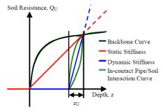
Fig. 2.4 Three soil stiffness
