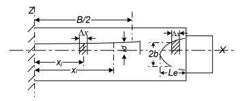
Fig. 7. Flattening between the upper and down work rolls
