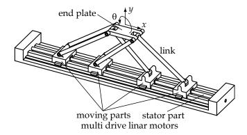
Fig. 3. Schematic view of the 3D4M mechanism
