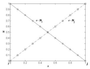
Fig. 2. Linear shape functions
