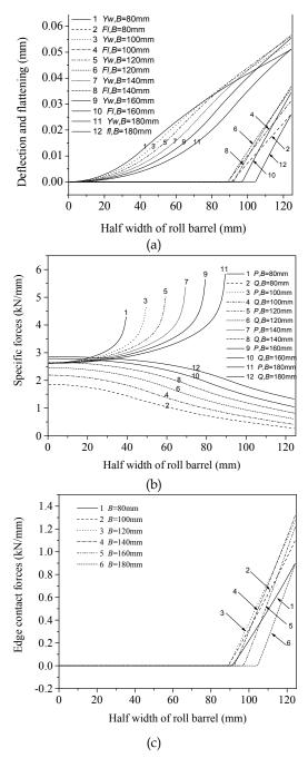
Fig. 13. Effect of the strip widths on the roll deflection and flattening (a), specific forces (b) and edge contact forces (c)
