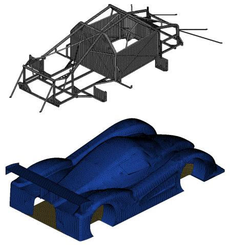
Fig. 14. Mesh of the E-Sphyra's frame and bodywork
