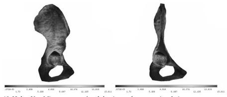
Fig. 18. Huber Von Mises eq. stress for abduction and cross-sectional view
