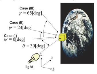
Fig. 10. Experimental conditions for the CCD camera location
