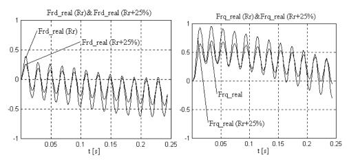
Fig. 2. Evolution of the flux orthogonal components with rotor resistance variation (low speeds).
