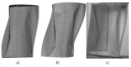
Fig. 27. Post-buckling deformation patterns under the same load:
