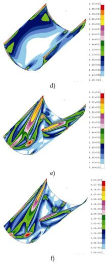
Fig. 30. Stress distributions according to Mises' hypothesis: (a model with stringers represented by beam elements): d) 25% load — external layer; e) 70% load — external layer; f) 100% load — external layer.
