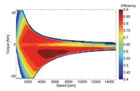
Fig. 8. Example of synchronous electric motor efficiency map.
