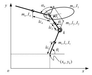
Fig. 1. A novel mechanism for one-legged hopping robot
