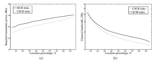
Fig. 7. (a) Required transmitter power to achieve a BER $< 10^{-9}$  and (b) channel bandwidth as a function of the receiver location percentage.
