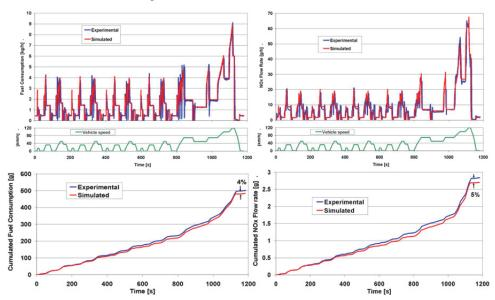
Fig. 4. Top: fuel consumption and NOx emission rate over warm NEDC cycle for a conventional powertrain. Bottom: cumulated fuel consumption and NOx emissions on the same driving cycle (from Vassallo et. al., 2007).
