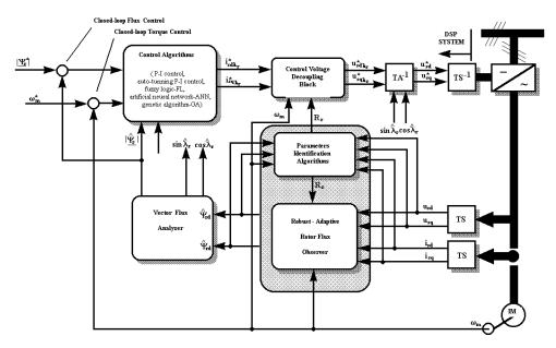
Fig. 7. Vector control of induction motor with speed rotor measurement [8].
