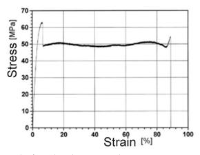
Fig. 17. Tensile stress plot for polycarbonate sample
