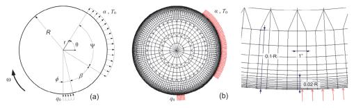
Fig. 8. (a) Thermal load configuration analyzed; (b) plane FE model (global and zoom)
