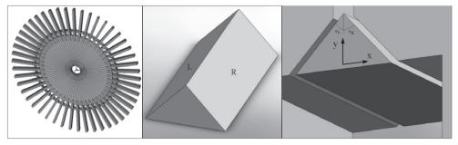
Fig. 21. Blisk geometry, damper geometry and damper location under the blade platforms.
