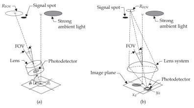
Fig. 1. (a) Conventional single-channel receiver (CSCR). (b) Single-channel imaging receiver (SCIR). The CSCR employs a lens in conjunction with a single photodetector. The SCIR employs an imaging lens system combined with a small photodetector placed on a miniaturized positioning mechanism.
