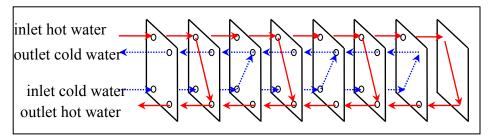
Fig. 1. Schematic presentation of counter flow plate heat exchanger with eight thermal plates
